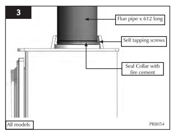
2.2 Connect a flue pipe 612mm long by inserting it into the flue spigot and seal using fire cement. Fit the cast iron finishing collar over the flue pipe and locate into recess in the top cover
